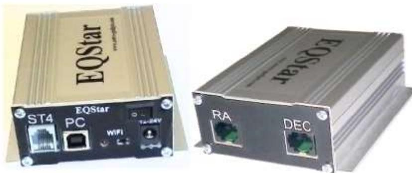
EQStar Inputs, Outputs, and Control
