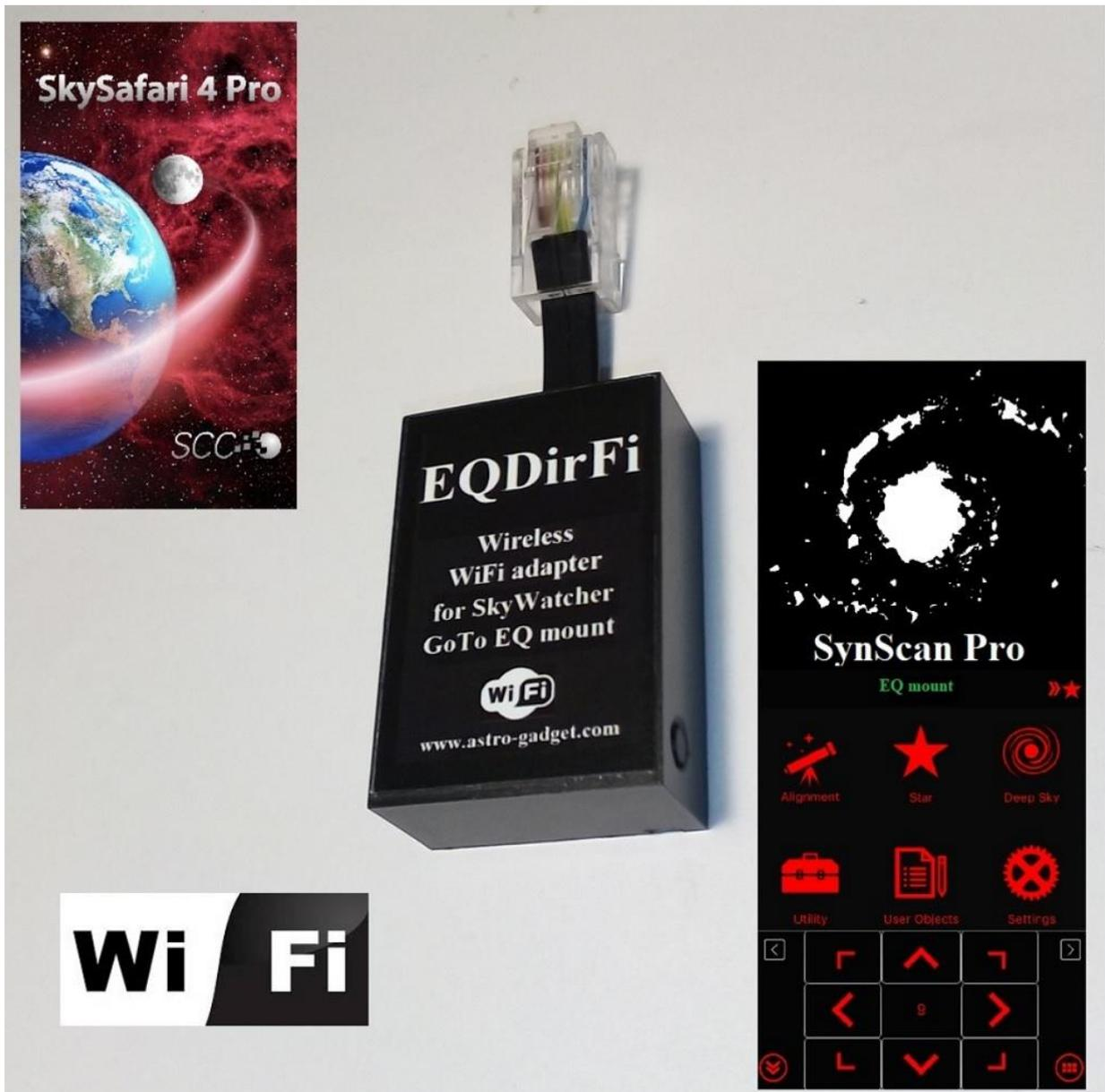
**EQDirFi**- is a wireless WiFi adapter for direct control of equatorial mounts SkyWatcher, ORION. Connect EQDirFi instead of the manual controller SynTrek or SynScan and get wireless GoTo !!! WiFi module operates only in access point mode!
